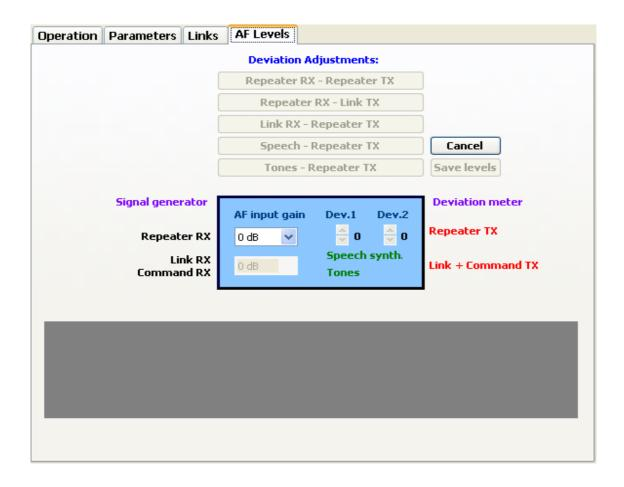
Click the button for the adjustment you want to perform. There is a on-screen instruction on how to connect the test equipment.
