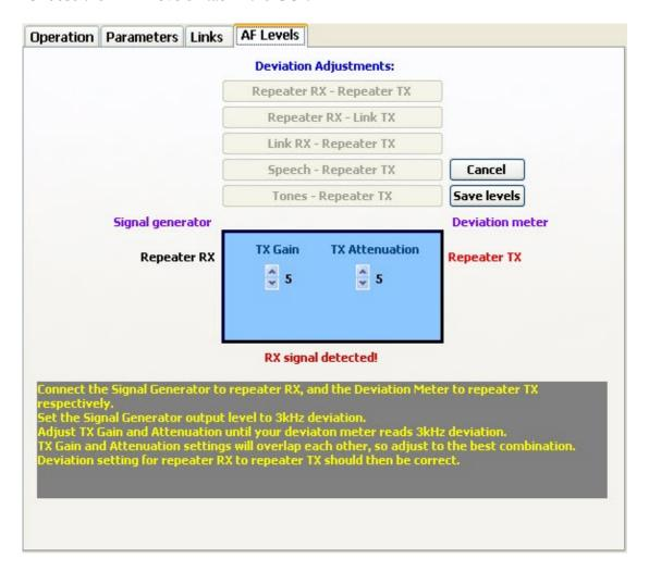
There you will find several buttons, and click the button for the adjustment you want to perform. There is a on-screen instruction on how to connect the test equipment.
